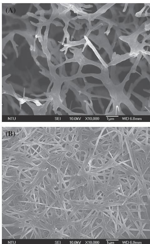
**Figure 2.** SEM images of hydrogels (A) **G1** and (B) **G2**.
